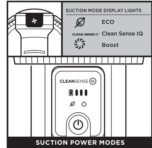
Press the button to toggle between ECO, Clean Sense IQ, and Boost modes. To save battery power, select ECO mode. For everyday cleaning power, select Clean Sense IQ mode. For an extra burst of power, select Boost mode.
