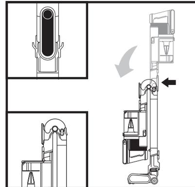
To put the vacuum in storage mode, press the unlock latch while folding the handheld vacuum forward.
