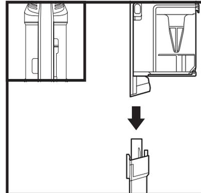
Press the Wand Release button at the top of the wand to detach the handheld vacuum.
