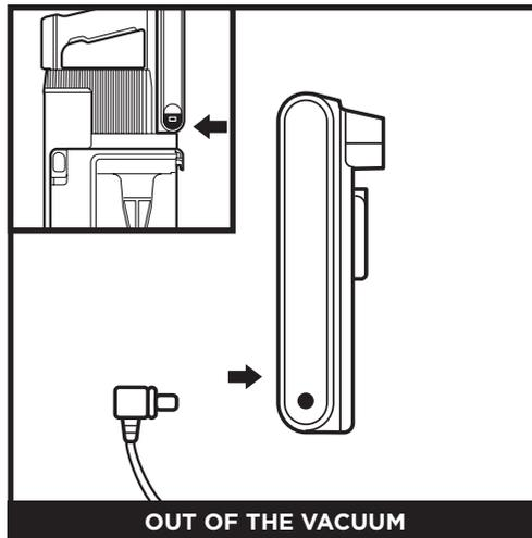
Press and hold the **Battery Release Button**, then slide out the battery. Plug the charger into the charging port on the battery. To reinstall the battery, slide it into the slot in the back of the handheld vacuum.
