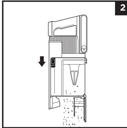
To empty the **Dust Cup** while it is attached to the handheld vacuum, position the dust cup over a trash receptacle and slide the **CleanTouch™ Dirt Ejector** slider forward.
