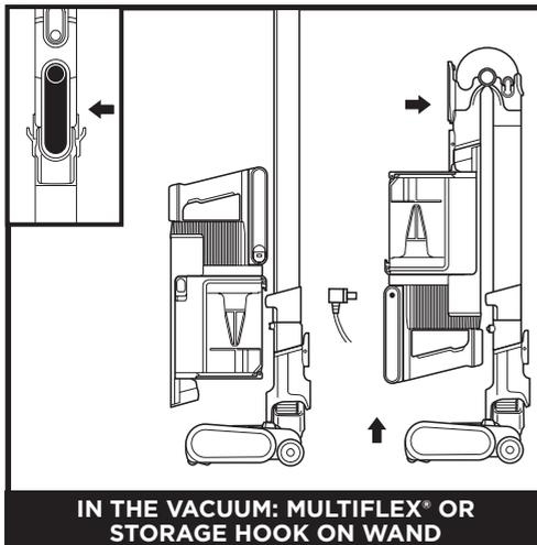
To store the vacuum for charging, press the **MultiFLEX Wand Unlock Latch** while folding the handheld vacuum forward until the wand clicks and locks, or hang the handheld vacuum from the storage hook on the wand. Plug the charger into the charging port on the handheld vacuum.
