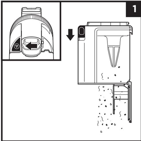
To remove the dust cup from the handheld vacuum, press the **CleanTouch Dust Cup Release** button near the handheld vacuum nozzle. Tilt the dust cup and lift off to remove. To empty dust and debris, hold the dust cup over the trash receptacle, then slide the **CleanTouch Dirt Ejector** slider forward.
