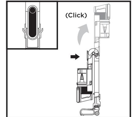
To take the vacuum out of storage mode, press the unlock latch and lift up the handheld vacuum until the wand clicks and locks into place.
