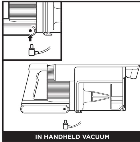
To charge the battery inside the handheld vacuum, connect the charger to an electrical outlet, then insert the charger plug into the port below the handle on the handheld vacuum.
