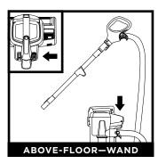
Press the **Wand Release** button and pull up on the wand to detach it from the pod.
