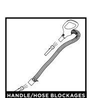
Detach handle from wand and hose from the vacuum pod, and check openings for blockages.
