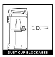
Detach dust cup from vacuum pod. Empty dust cup, remove debris from lint screen, and check for blockages.
