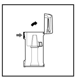
To remove collected debris from **Lint Screen**, press top release button and lift handle to open. Gently brush lint screen to clean.
