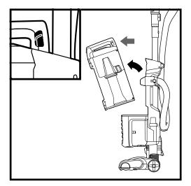
To remove **Dust Cup**, slide up the release button on the dust cup handle. Tilt dust cup forward, then lift to remove.
