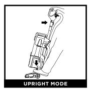
Press the Power/Surface switch to the appropriate floor setting, then step on the nozzle and tilt the handle back to engage the brushroll.
