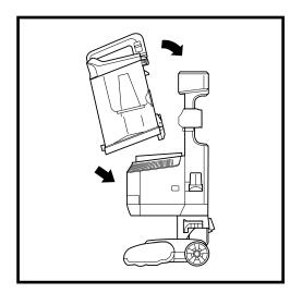
To reinstall, place the bottom of the dust cup onto the pod and then tilt until it clicks into place.
