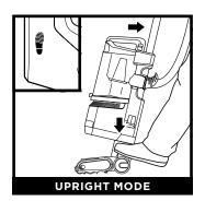
To engage Brushroll, step on floor nozzle and tilt handle back firmly.
