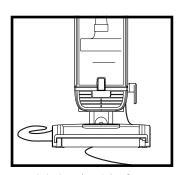
To minimize the risk of power cord damage, **DO NOT** run the vacuum over the power cord. If this occurs, immediately shut off power to the vacuum and remove the cord from the brushroll or nozzle.
