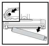
Slide the Soft Roller access button forward to release the Soft Roller.
