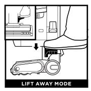
Step on the pedal on the floor nozzle to lift off the pod.
