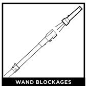
Detach wand from pod and handle, and check both ends for blockages.
