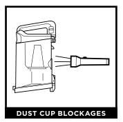
Detach dust cup from vacuum pod. Empty dust cup and remove debris from lint screen in the top of the dust cup.
