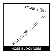
Detach hose from handle by pressing on the release button at the top of the hose. Detach the hose from the pod, and check openings for blockages.
