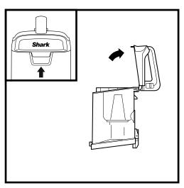
Clear debris from the **Lint Screen** in the dust cup. Lift the upper release tab at the top of the dust cup and open the lid. Gently brush the lint screen to remove debris.
