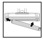
Hand wash the Soft Roller as needed. Use only water, and allow it to air-dry completely for at least 24 hours. Reinsert the Soft Roller in the front of the nozzle until it clicks into place.
