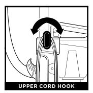
For cord access, rotate upper hook down and remove cord.
