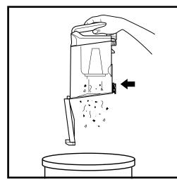
To empty debris into the trash, press the lower release button and the bottom of the dust cup will drop open.
