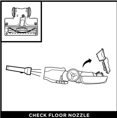
Detach the wand. Turn the floor nozzle over and use the edge of a coin to open the three locks on the bottom of the floor nozzle.
