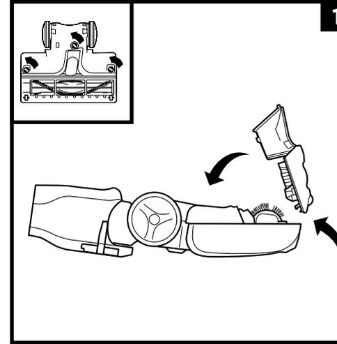
To access the brushroll, flip the floor nozzle over and use the edge of a coin to open the three locks on the bottom of the floor nozzle.
