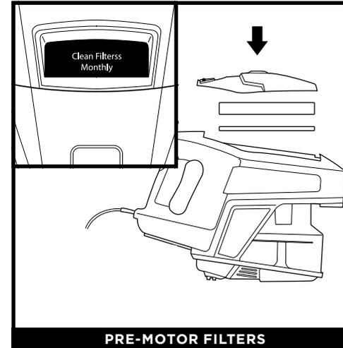
Open the lid on the top of the handheld vacuum to lift out the pre-motor filters. The **Pre-Motor Filters** should be washed once a month.
