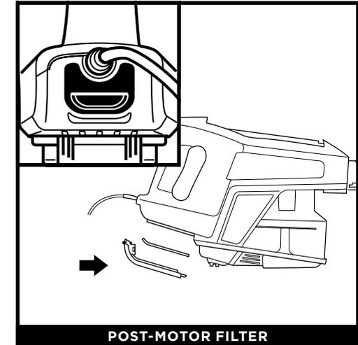
To remove the post-motor filter, open the filter cover on the handheld vacuum and pull out the filter. The **Post-Motor Filter** should be washed once every year.
