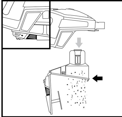
To remove the dust cup from the handheld vacuum, squeeze the two **Dust Cup Release** buttons at the same time and pull out the dust cup. Hold the dust cup over the trash, then press the Empty button to release dirt and debris.
