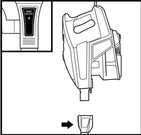
Press the **WAND RELEASE** button and lift the handheld vacuum off the wand.
