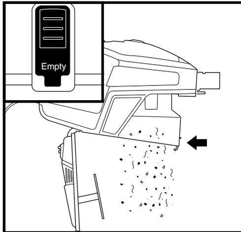
With the dust cup attached to the handheld vacuum, hold the handheld vacuum over the trash, then press the Empty button on the dust cup to release dirt and debris.
