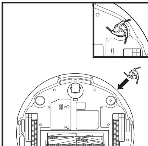
Snap the 1 included **Side Brush** located in the red packaging, onto the square peg on the bottom of the robot.
