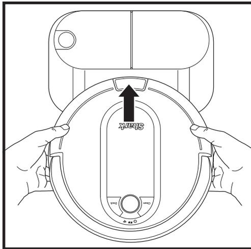
If the robot has no charge and cannot return to the base, manually place it on the base. When the robot evacuates dust and debris into the base, the blue light on the base will be solid blue. Once charging starts, the robot will beep and the blue light on the base will pulse.
