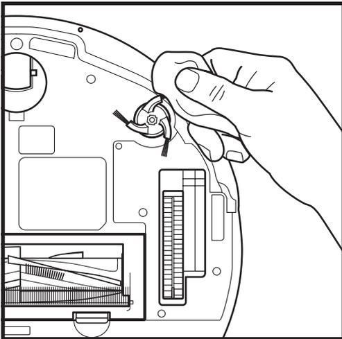
Carefully unwind and remove any string or hair wrapped around brush.
