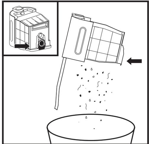
To empty the bin, hold it over the trash, then press the release button with the trash can icon on the bottom of the bin. The bin lid will open, releasing dust and debris. Lightly tap the dust bin against the inside of the trash receptacle to knock off any remaining debris. Reinstall the bin by sliding it into the slot in the base until it clicks into place.
