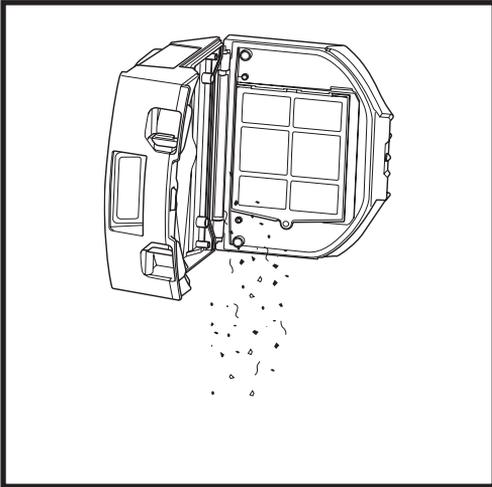
Empty debris and dust into trash.
