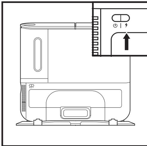
When charging begins, the robot will beep. The **BLUE Charging Indicator Light** on the base will **PULSE**, and the **Battery Indicator Light** on the robot will flash blue. When the robot is fully charged, the battery light on the robot and the blue charging indicator light on the base will illuminate steadily.
