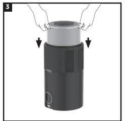
**3.** With the filter reinstalled, twist the filter door until it clicks into place.
