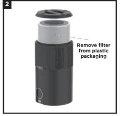
Take the filter out of its packaging, then insert it back into the unit.
