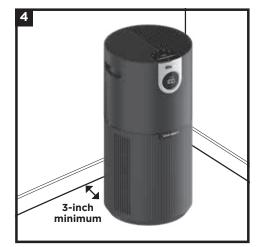
4 Set up the unit on a level surface, at least 3 inches (8-cm) away from walls and objects.
