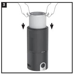
**3.** With the filter reinstalled, twist the filter door until it clicks into place.
