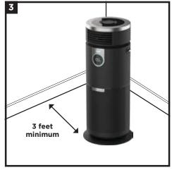
**3.** Set up the air purifier up at least 3 feet (0.9m) from the wall and any furnishings. Plug it in and power on.
