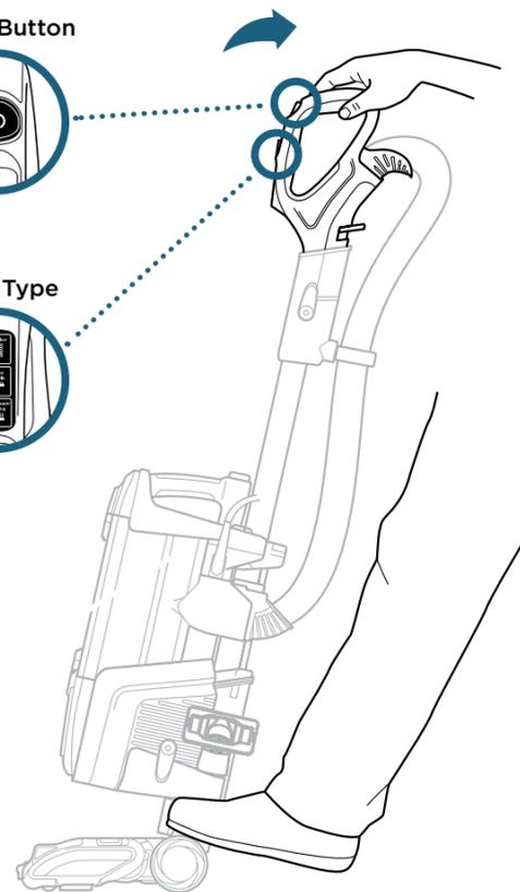
Place foot on floor nozzle and tilt handle back. Choose appropriate floor setting and press power button.
