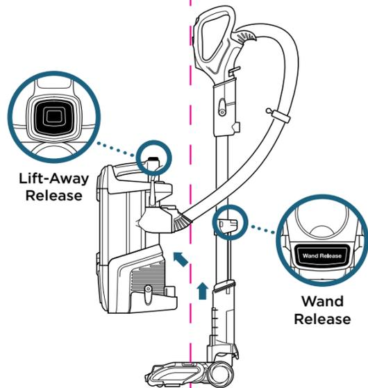
Press Lift-Away Release button to lift pod off floor nozzle. You are now ready to clean those hard-to-reach places.
