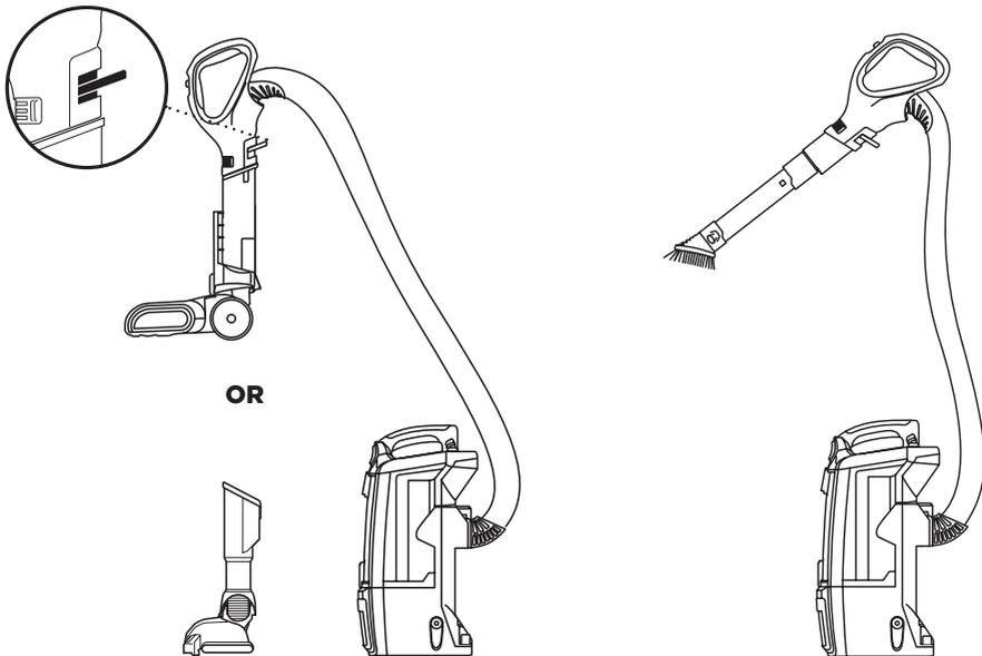
**2** Insert handle into either the motorized floor nozzle or the Dust-Away™ Pro. Now you have a convenient way to clean stairs.
