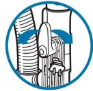
For quick cord access, rotate upper hook down and remove cord.
