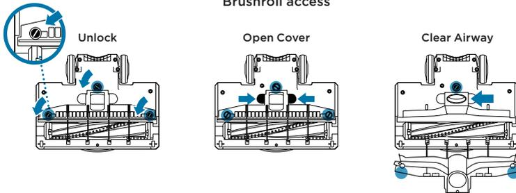
Using a coin, turn locks counterclockwise to open, then lift off cover to access brushroll.
