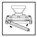
Hand wash the Soft Roller as needed. Use only water, and let air-dry completely for at least 24 hours. Reinsert the Soft Roller under the rubber bumper in the front of the nozzle until it clicks into place.
