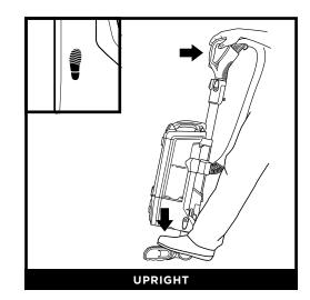
To engage brushroll, turn power on, select a surface setting, then place foot on floor nozzle and tilt handle back.
