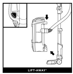
Press Lift-Away button to lift pod off motorized floor nozzle. You are now ready to clean those hard-to-reach places. Attach cleaning tools directly to the handle or to the wand for extended reach.
