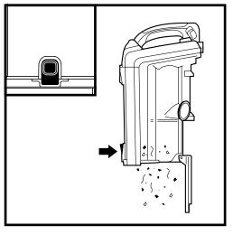
Hold dust cup over a trash bin and press the empty-release latch on the bottom to empty dust and debris into trash.
