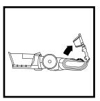
Lift up the lid on the bottom of the nozzle to access the brushroll. Use a flashlight to check for blockages.
