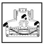
Use the edge of a coin to open the 3 locks on the bottom of the floor nozzle.
