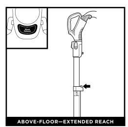
Press the **Wand Release** button to detach the wand to clean with more reach. Insert cleaning tools directly into wand or handle.
