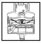
With scissors, carefully cut along the groove in the brushroll to remove any debris, hair, or fibers.
