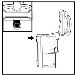
Press top dust cup release latch to access dust screen and remove built-up debris as necessary.
