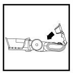
To reinstall the lid, line it up along the front of the nozzle and press it closed. Use the coin to close the 3 locks.
