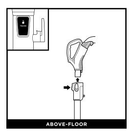
Press the **Handle** button to detach the handle to clean above-floor areas or with attachments. Insert cleaning tools directly into wand or handle.
