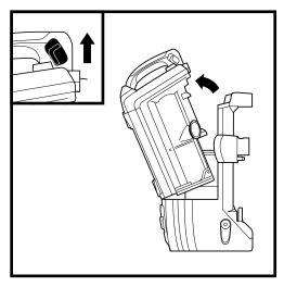
Pull up on **Dust Cup**, release latch and lift dust cup off pod
