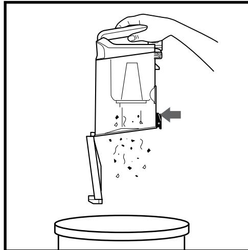
Hold the dust cup over the waste bin and press the release button to open bottom of dust cup.
