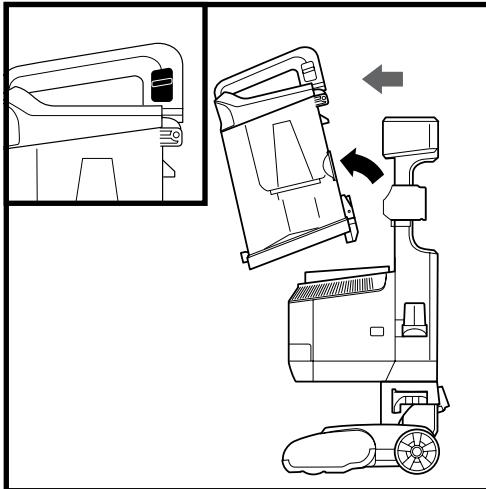
To remove **Dust Cup**, pull up on the release button located on the side of dust cup handle. Tilt dust cup forward, then lift to remove.
