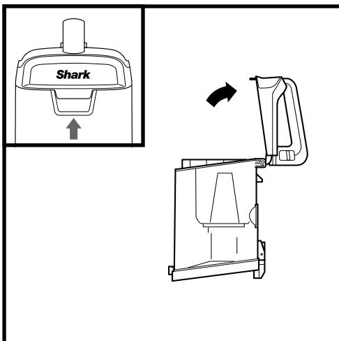
To remove collected debris from **Lint Screen**, lift the tab at the top of the dust cup to open the lid. Remove debris from lint screen to clean.
