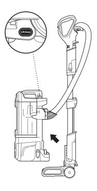
1 Press Lift-Away® button to lift pod off motorized floor nozzle.
