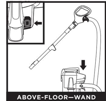
Press the **Wand Release** button and pull up on the wand to detach it from the pod.
