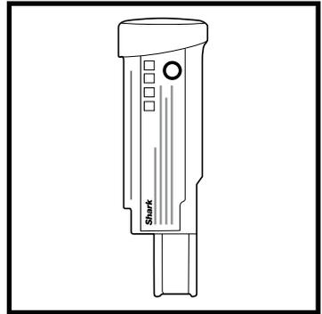
2. Press the cap until the battery clicks securely into place.
