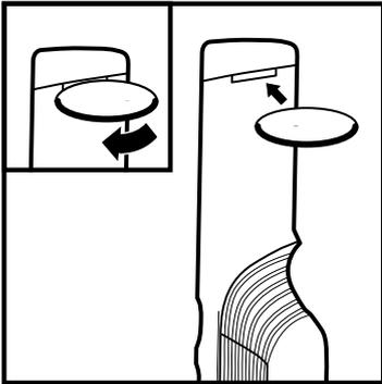
2. Gently pull the cap to slide out the battery. Set the battery on a level surface.
