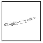
Detach wand from floor nozzle and remove brush roll cover. Tilt nozzle neck back to straighten the airway, and remove any blockages.
