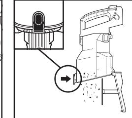
bottom button to release dust and debris.
