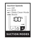
Press the (+) button to togale between ECO. Deep Clean and Boost modes. To save battery power, select ECO mode. For everyday cleaning power, select Deep Clean Mode, For an extra burst of power, select Boost mode.
