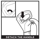
To clean above-floor areas close at hand, press the Handle Release trigger to detach the handle from the wand.
