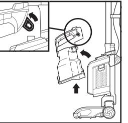
To remove **Dust Cup**, slide up the release tabs on both sides. Tilt the dust cup away from pod, and lift to remove.
