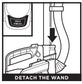
Detach the wand from the pod for more reach to clean above-floor areas. Press the Wand Release button and lift the wand to remove it from the nozzle.
