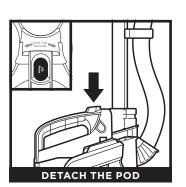
Detach the pod from the floor nozzle for powerful cleaning under furniture and in other hardto-reach areas. Press the LIFT-AWAY button and lift the pod off the nozzle.
