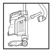
Detach hose from vacuum pod, and check opening on back of pod for blockages.
