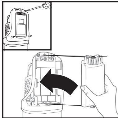
1. If the battery pack cover is installed on the handheld vacuum, remove the 4 screws on the cover with a Phillips-head screwdriver and lift off the cover.
