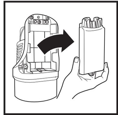
4. Lift the battery out of the housing.
