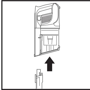
1. Remove the handheld vacuum from the wand by pressing the wand release button and pulling up.
