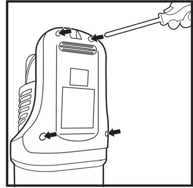
2. Use a Phillips-head screwdriver to remove the 4 screws on the battery pack cover on the bottom of the handheld vacuum.
