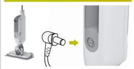
Plug the **charger** into an electrical outlet, then insert the charger plug into the port on the back of the main body. The unit will begin charging.
