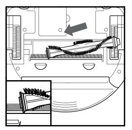
Install the brushroll in the replacement robot, inserting the flat end first. Close the brushroll access door and press down until it clicks into place.
