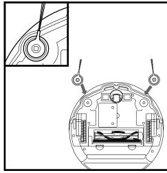
Remove the 2 side brushes from your original unit by pulling them off the pegs on the bottom of the robot. Install them on the replacement robot by pressing them down over the pegs until they click into place.
