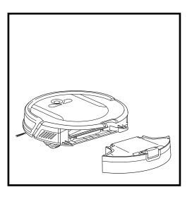
Press the dust bin removal button on your original robot, and slide out the dust bin. Slide the dust bin into the replacement unit.
