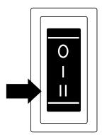
**2** Press the Power/Surface switch to setting I to vacuum bare floors. The brushroll will not spin in this mode.
