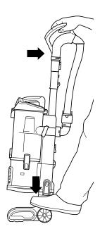
Plug power cord into outlet. Place foot on floor nozzle and tilt handle back. STEP 2
