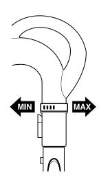
2 Attach an accessory onto the end of either 3 The Suction Control slider is located at the base of the handle. Slide clockwise for more suction, or counterclockwise to reduce suction.
