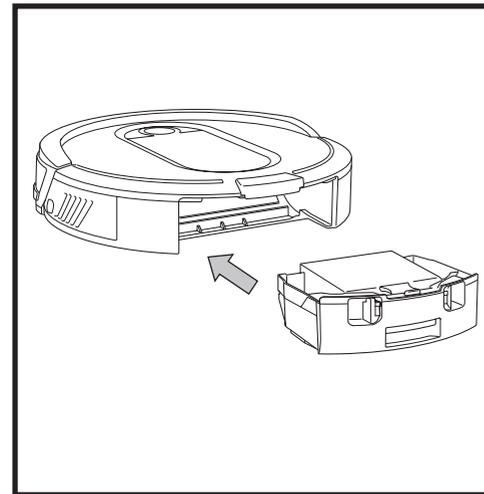
Reinsert the filter into the robot dust bin, then slide the dust bin back into the robot.
