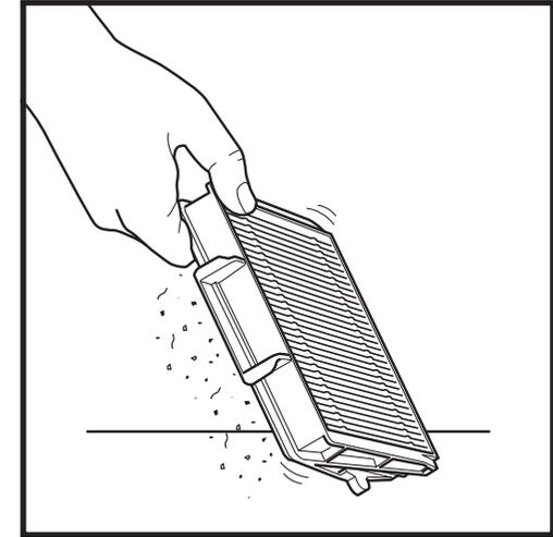
Lightly tap the filter to remove dust and debris.
