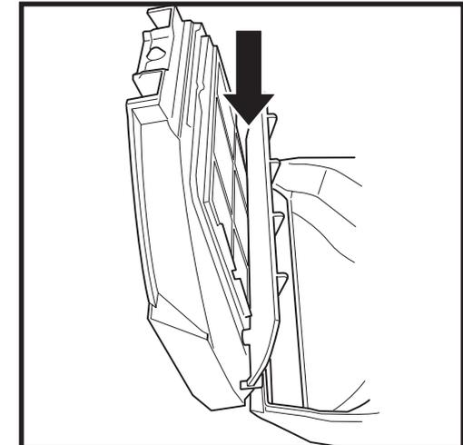
Look between the filter and plastic shield and make sure there is no debris buildup.
