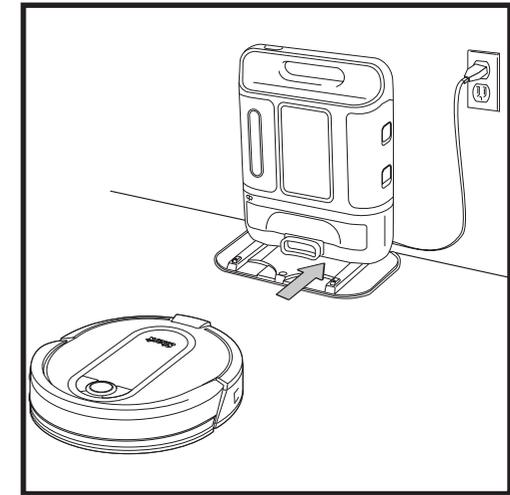
When charging begins, the robot will beep. The **BLUE Charging Indicator Light** on the base will **PULSE**, and the **Battery Indicator Light** on the robot will flash blue. When the robot is fully charged, the battery light on the robot and the blue charging indicator light on the base will illuminate steadily.
