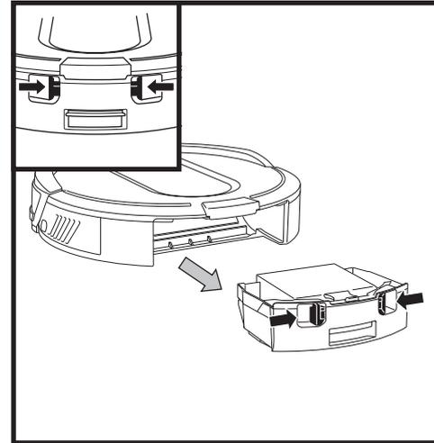
Press the **Dust Bin Release Tabs** and slide out the dust bin.
