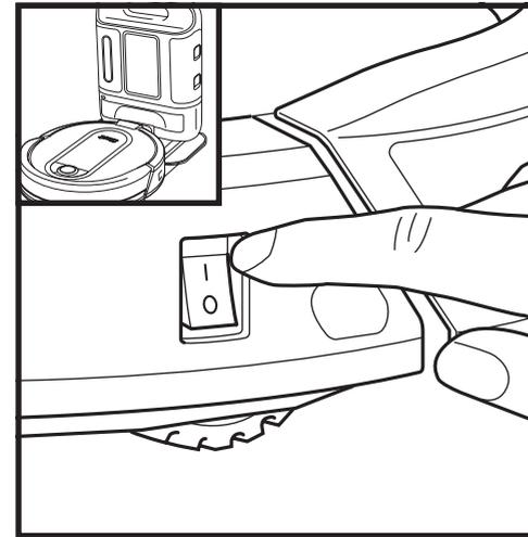
To charge, place the robot with its **BACK** side against the base. The metal **Charging Pads** on the bottom of the robot must be touching the **Charging Contacts** on the base. Make sure the power switches on **BOTH** the robot and the base are turned to the (I) ON position.
