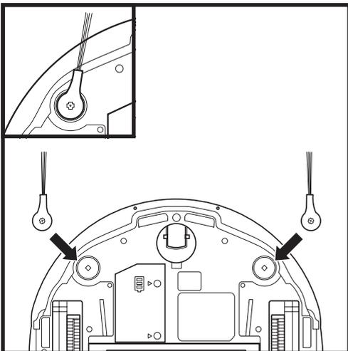
Snap the 2 included **Side Brushes** onto the square pegs on the bottom of the robot.
