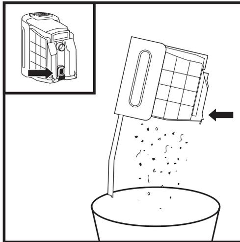
To empty the bin, hold it over a trash can and press the **Empty** button on the side.
