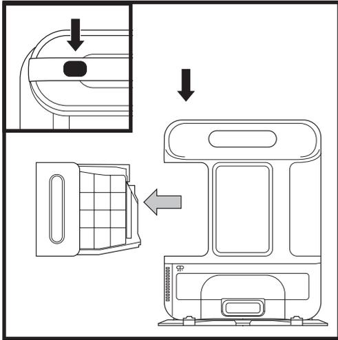
The **Base Dust Bin** holds up to 45 days' worth of dust and debris. Empty the bin when the debris level approaches the max fill line.
