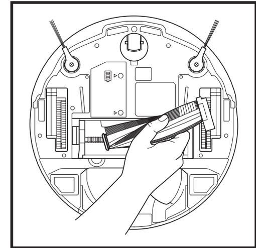
Lift out the brushroll, and clean off any debris. Reinstall the brushroll, inserting the flat end first. Close the brushroll access door and press down until both sides click into place.
