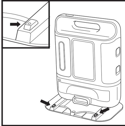
**IMPORTANT:** The robot uses cliff sensors to avoid stairs and other steep drops. Sensors may work less effectively when they are dirty. For best results, clean sensors regularly.
