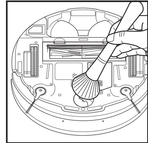
Clean the wheel housing, then reinsert the caster wheel.
