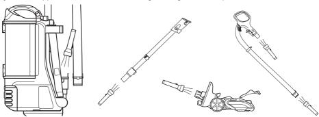
Detach hose from vacuum pod, and check hose and opening on back of pod for blockages.
