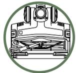
**NOTE:** If you see any hair wrapped around the brushroll, continue cleaning, using Setting II, Carpet, on bare floors. This will allow Zero-M™ technology to remove the hair wrap and send it to the dust cup.
