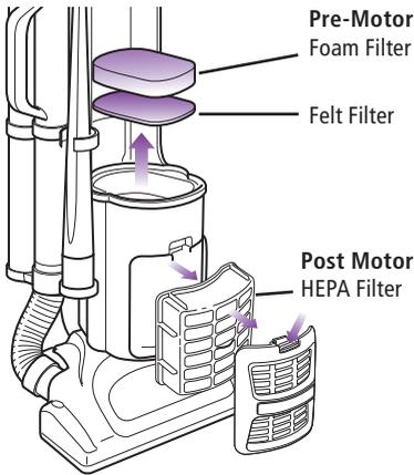
**⚠ IMPORTANT: Loss of Suction may occur** if foam filter is not cleaned every month. Rinse and allow to air dry completely. Also, tap loose dirt off filter between washes as needed. Foam filters may appear dirty after use - this is normal.
