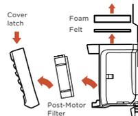
Remove dust cup to access foam and felt filters. Next, press down top of filter door. Tilt filter door and lift out. Press tab at top of HEPA filter and pull away from the base of the vacuum.
