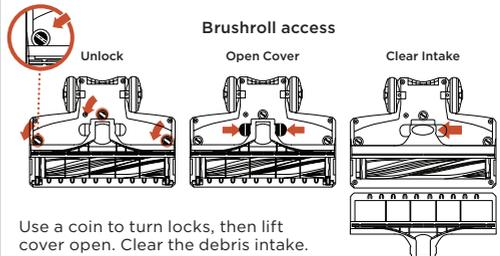
Use a coin to turn locks, then lift cover open. Clear the debris intake.
