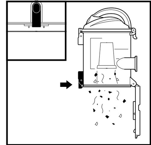
Press lower release button to open bottom of dust cup.
