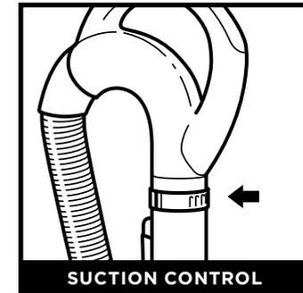
The **Suction Control Slider** on the handle allows you to adjust the suction depending on the floor type.
