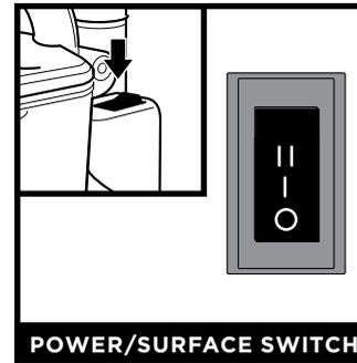
Press the Power/Surface Switch at the top of the pod.
