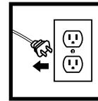
**IMPORTANT:** Unplug the power cord before performing any maintenance. Empty the dust cup each time you vacuum and periodically during cleaning, when debris in the dust cup reaches the MAX fill line.
