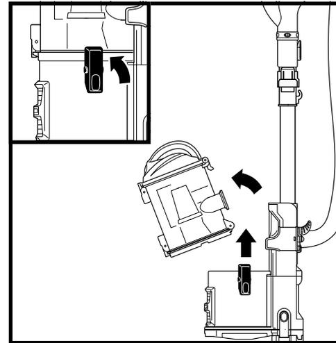
To remove **Dust Cup**, slide up tabs on both sides of dust cup. Tilt dust cup forward, then lift to remove.
