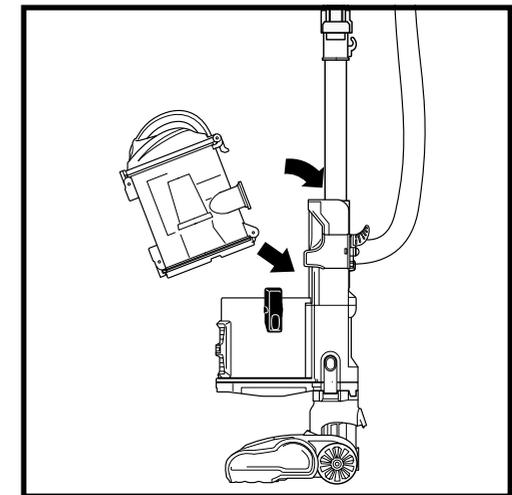
To reinstall, place bottom of dust cup into pod first and pull the latches down to lock in place.
