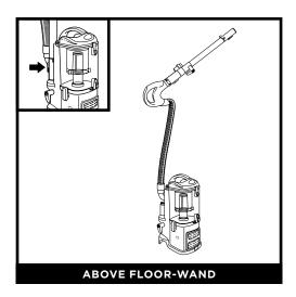
Follow instructions for detaching the pod above. Press the **Wand Release** button to remove the wand from the pod. Attach an accessory to the end of the wand.
