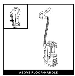
Follow instructions for detaching the pod and wand. Press the **Handle Release** button to detach the handle from the wand. Attach an accessory to the end of the handle.
