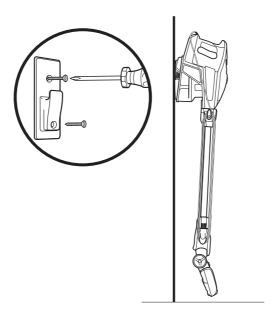
**2** Use the wall mount that is included. Drill two 5/16" holes and insert plastic anchors provided into the wall. Using a Philips head screwdriver, screw the wall mount into the plastic anchors. Hook the catch on the bottom of the handheld vacuum onto wall mount.
