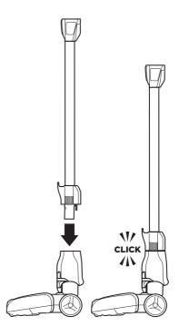
1 Insert the wand into the motorized floor nozzle connector until you hear a click.
