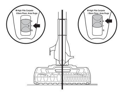
The Rocket® Ultra-Light has a 2-speed Power slider switch on the handle. Slide the Power switch to appropriate speed setting (I or II) and start cleaning.
