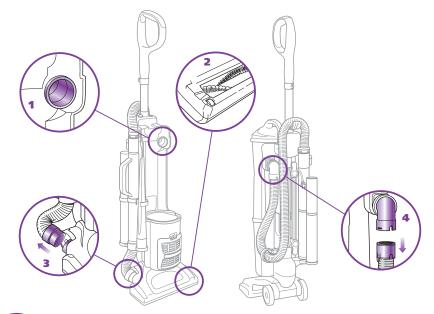
Unplug the vacuum before checking for blockages.
