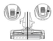
Bare Floor, Area Rugs (I) - The brushroll and the Soft Roller both spin together slowly to clean bare floors and area rugs. The Soft Roller traps fine dust and large particles, while the brushroll directs that debris to the suction channel.
