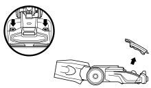
2 Lift the brushroll out by the tab on the left side. Use a pair of scissors to carefully remove any string, hair or debris that may be wrapped around the brushroll.
