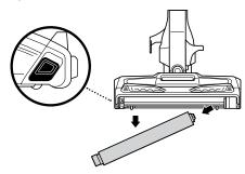
Remove any string, carpet fibers or hair that may be wrapped around the Soft Roller. You can also tap loose debris off the Soft Roller, or wipe it clean with a dry towel. If you see any fibers or hair buildup in the teeth behind the Soft Roller, take a dry towel and wipe it away.
