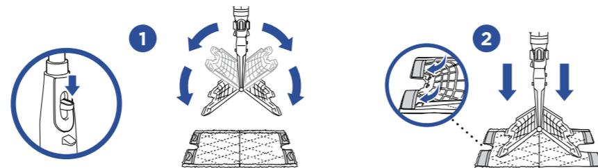
1. Lift the mop straight up by the handle until the Genius Mop Head is hanging straight down. Center the Genius Mop Head above the pad. Press the pad release button, and both sides of the mop head will drop open.
