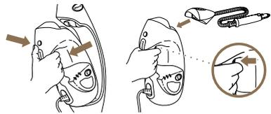
Once done with handheld steaming, press the **STEAM CONTROL** button until the light flashes blue to put the unit in **STANDBY MODE**. Let cool for 2 to 3 minutes before removing mop head, pads, or handheld accessories and storing.
