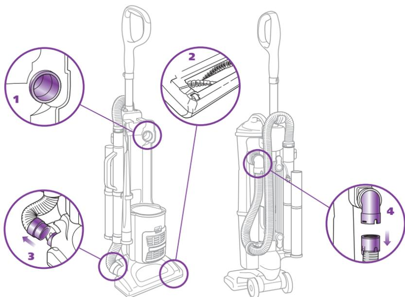
Unplug the vacuum before checking for blockages.
