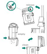
Rinse pre-motor filters every 3 months and HEPA filter once a year. Rinse with water only. Allow filters to air-dry completely before reinstalling.
