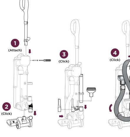
Attach handle assembly to vacuum body with screw, then connect body to motorized floor nozzle.
