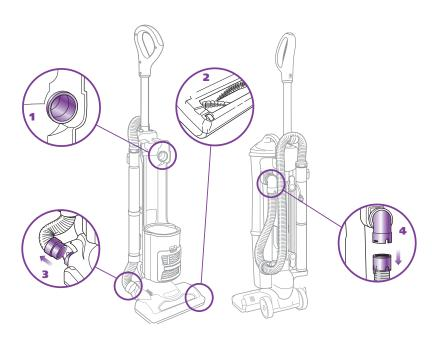
Unplug the vacuum before checking for blockages.
