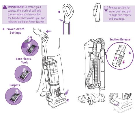
Your **Shark® Navigator®** Vacuum can be used to clean bare floors or carpets – with the click of a switch. Stand the vacuum into the upright position.
