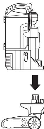
**1** Place the pod onto floor nozzle.
