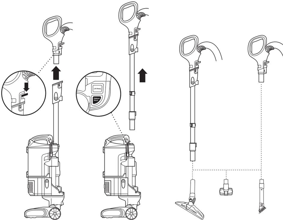
**2** Press the Wand Release button to release the wand. To release the handle only, push the handle latch down and lift handle up.
