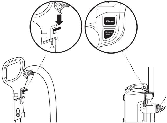
**1** To clean within short reach, push handle latch down, then lift the handle up off of the wand.
