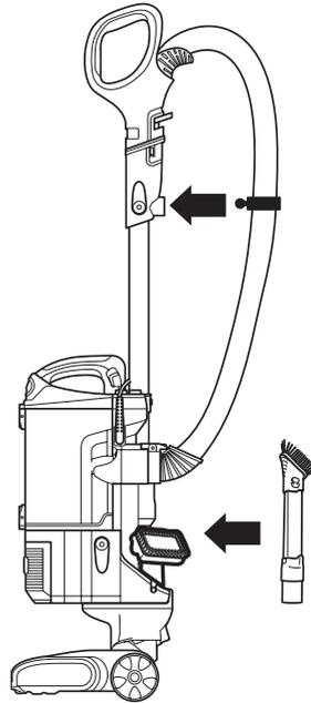
**3** Insert handle into top of wand. Then attach hose to hose connector on base of pod.
