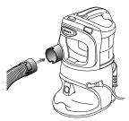
Insert the end of the flexible hose into the connector on the front of the Portable Vacuum. You will hear a "click" when it is in place. **STEP 2**
