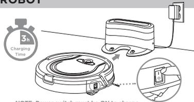
NOTE: Power switch must be ON to charge.
