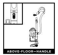
Press the **Handle Release** button and pull up on the handle to detach it from the wand.
