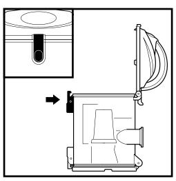
To remove collected debris from **Lint Screen**, press top release button and lift handle to open. Gently brush debris off the screen.
