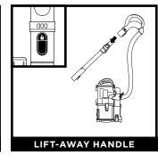
Press the **Handle Release** button and pull up on the handle to detach it from the wand.
