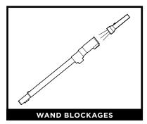
Detach wand from floor nozzle and handle, and check both ends for blockages.
