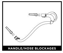
Detach handle from wand and hose from the vacuum pod, and check openings for blockages.
