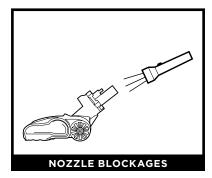
Detach floor nozzle from wand and vacuum pod, tilt nozzle neck back, and check opening for blockages.
