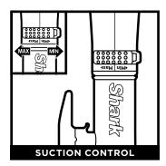
The **Suction Control Slider** located on the handle allows you to adjust the suction depending on the floor type.
