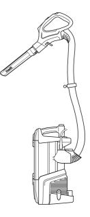
2 For a convenient way to clean stairs, detach wand and handle, then insert handle into motorized floor nozzle.
