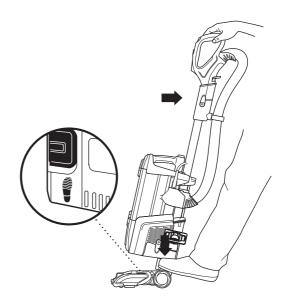
Plug power cord into outlet. Place foot on floor nozzle 1 and tilt handle back.
