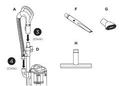
Connect handle to the wand, pressing until it clicks into place. Connect hose to the back of the canister pressing until it clicks into place.
