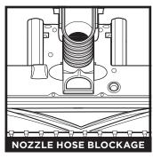
To access the nozzle hose, pinch the release touchpoints on the bottom of the nozzle, then lift the cover and clear any blockages.
