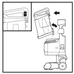
To remove the **Dust Cup**, slide up on the release button located on the side of dust cup handle. Tilt dust cup forward, then lift to remove.
