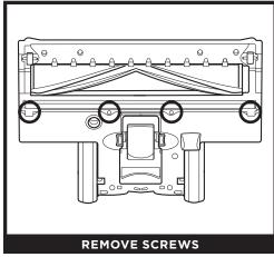
1. Turn the nozzle over and locate the squeegee bristle strip between the brushroll and the rear wheels. Use a Phillips-head screwdriver to remove the 4 screws.
