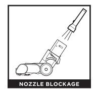
Detach wand from floor nozzle, tilt nozzle neck back, and check opening for blockages.
