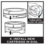
Align the yellow arrow on the side of the cartridge with the yellow arrow on the side of the dial cover, then insert the cartridge into the dial. Rotate the cartridge clockwise to lock it in place.
