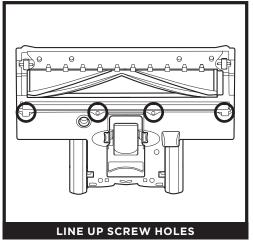
2. Align the 4 screw holes on the squeegee strip over the holes in the nozzle. Make sure the strip sits flush with the nozzle, then fasten it securely in place with the screws.
