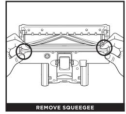
2. Remove the squeegee strip by pulling up on the fabric flaps on both ends of the strip.
