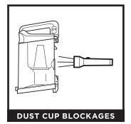
Detach dust cup from vacuum pod. Empty dust cup and remove debris from lint screen in the top of the dust cup.
