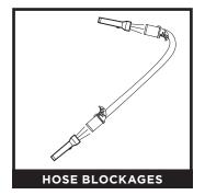
Detach hose from handle by pressing on the release button at the top of the hose. Detach the hose from the pod, and check openings for blockages.
