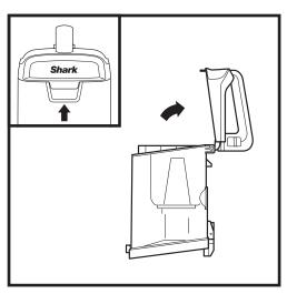
Clear debris from the **Lint Screen** in the dust cup. Lift the upper release tab at the top of the dust cup and open the lid. Gently brush the lint screen to remove debris.
