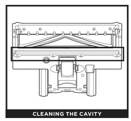
With the strip removed, clean the squeegee cavity and bristle strip. Use a paper towel to wipe off any debris or dust in the cavity and on the bristle strip.
