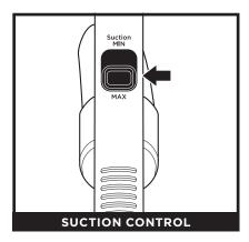
The **Suction Control Slider** located on the handle allows you to manually adjust the suction of your vacuum.
