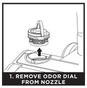
Flip up the handle and rotate the dial clockwise until the two teal arrows are aligned. Pull the handle to remove the dial from the nozzle.
