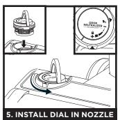
Align the teal arrow on the dial cover with the teal arrow on the nozzle, then reinsert the dial into the nozzle. Rotate the dial counterclockwise until it clicks into an intensity setting to engage. Rotate further to change the intensity setting.
