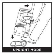
To engage the **Brushroll**, press the power button, select a surface mode, step on the floor nozzle, and tilt the handle back firmly.
