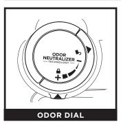
Flip up the dial handle and rotate the odor dial to adjust Odor Neutralizer Technology intensity or to unlock the dial for cartridge access.
