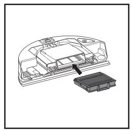
Reinsert the filter into the dust bin, then slide the dust bin back into the robot until it clicks into place.
