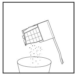
To empty the bin, hold it over the trash, then press the release button with the trash can icon on the side of the bin. The bin lid will open, releasing dust and debris. Lightly tap the dust bin against the inside of the trash receptacle to knock off any remaining debris. Reinstall the bin by sliding it into the slot in the base until it clicks into place.
