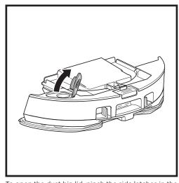
To open the dust bin lid, pinch the side latches in the finger slots and hold them while lifting the lid.
