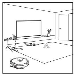
The robot's object detection technology helps it navigate around obstacles taller than 4.5" in height. Clear away small objects that may interfere with the cleaning path of your robot.
