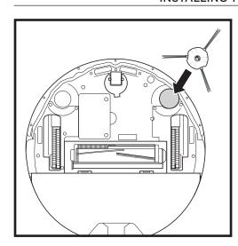
Snap the included long single side brush onto the square peg on the bottom of the robot. The brush will spin clockwise when correctly assembled.
