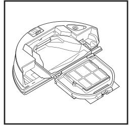
Look between the filter and the plastic shield and make sure there is no debris buildup.
