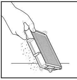
Lightly tap the filter to remove debris every time you empty the dust bin. Replace the filter every 6-12 months or as needed.
