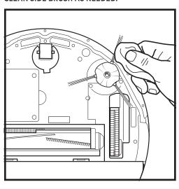
Carefully unwind and remove any string or hair wrapped around the long single side brush.
