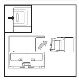
Depending on the size of the base, empty the base dust bin every 30 to 60 days or as needed.
