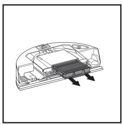
Remove and empty the Self-Empty Dust Bin. Pull filter out of the dust bin by the tabs.
