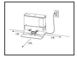
Place the Landing Mat on the floor and align the self-empty base on top so that it sets into place
