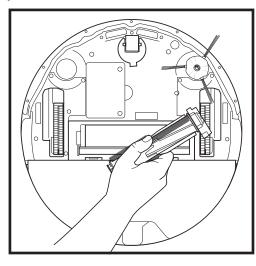
Lift out the brushroll and remove any debris. Remove the end cap to clean out any trapped hair or debris. Replace the end cap once clean.
