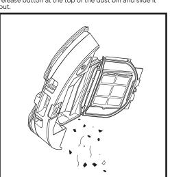
Remove the filter and use a damp cloth to wipe the dust bin clean. Allow the bin to air-dry for 24 hours before reinstalling it.
