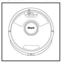
To turn ON the robot, press and hold the DOCK button for 5-7 seconds. To charge, place the robot on the base. The robot will beep when charging begins and the charging indicator on the base will illuminate.
