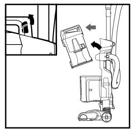
To remove **Dust Cup**, slide up the release button on the dust cup handle. Tilt dust cup forward, then lift to remove.
