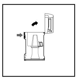
To remove collected debris from Lint Screen, press the top release button and lift the handle to open the dust cup. Gently brush lint screen to clean.
