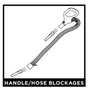
Detach handle from wand and hose from the vacuum pod, and check openings for blockages.
