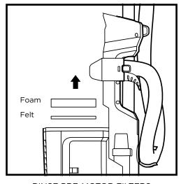
RINSE PRE-MOTOR FILTERS **EVERY MONTH** Remove **Dust Cup**, then lift out **Filters**.
