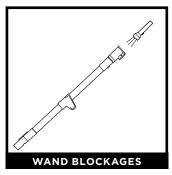
Detach wand from pod and handle, and check both ends for blockages.
