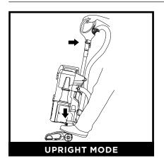
To engage **Brushroll**, turn on the power, step on the floor nozzle, and tilt handle back.
