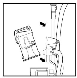
To reinstall, place the bottom of dust cup onto the pod and then tilt until it clicks into place.
