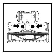
Using a coin, turn locks counterclockwise, then lift the cover to access brushroll.
