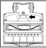
over a hard or sharp object or notice a noise change while vacuuming, check for blockages or objects caught behind the brushroll. Clear away any dust, dirt,
