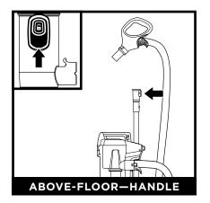
Press the **Handle Release** button and pull up on the handle to detach it from the wand. Attach an accessory to the handle.
