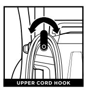
For cord access, rotate upper hook down and remove cord.
