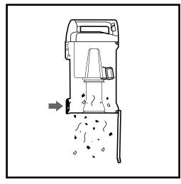
Press the release button to open bottom of dust cup.
