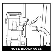
Detach hose from vacuum pod, and check hose and opening on back of pod for blockages.
