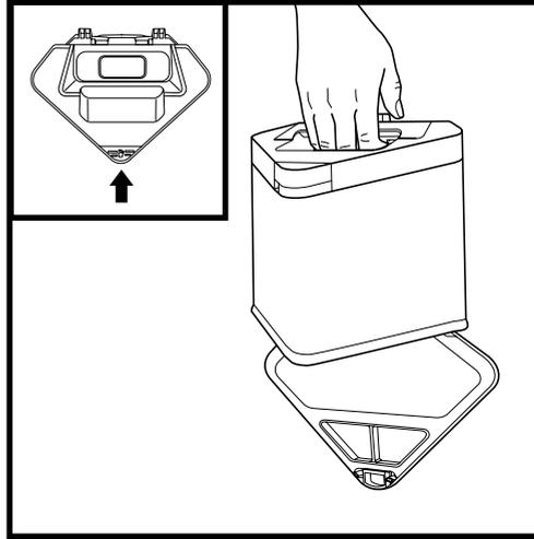
To empty the bin, hold it over the trash and press the release button on the top of the dust bin. The bottom will open to release the debris.
