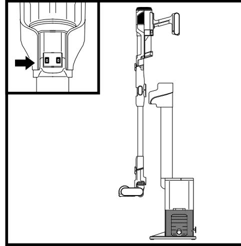
Place the vacuum on the dock with the wand in the cradle of the charging post. When the vacuum is properly docked, automatic evacuation will begin. The evacuation cycle will last for 15 seconds.
