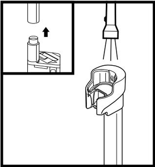
Checking for Blockages in the Charging Post:
