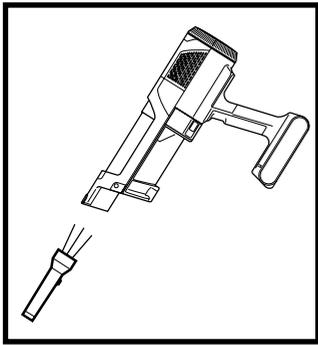
Checking for Blockages in the Hand Vacuum:
