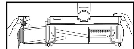
5. Tap off loose debris and wipe the brushroll clean with a dry towel. Hand wash the brushroll if needed, using only water, and then let it air-dry completely for at least 24 hours.
