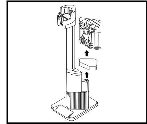
To access the Auto-Empty Exhaust Foam Filter, remove the dust bin. Before removing the Exhaust Foam Filter, vacuum off any fine debris from the surface. Lift the Exhaust Foam Filter out of the dock, then rinse it with water only (do not use soap). Allow the filter to air-dry completely before reinstalling it.
