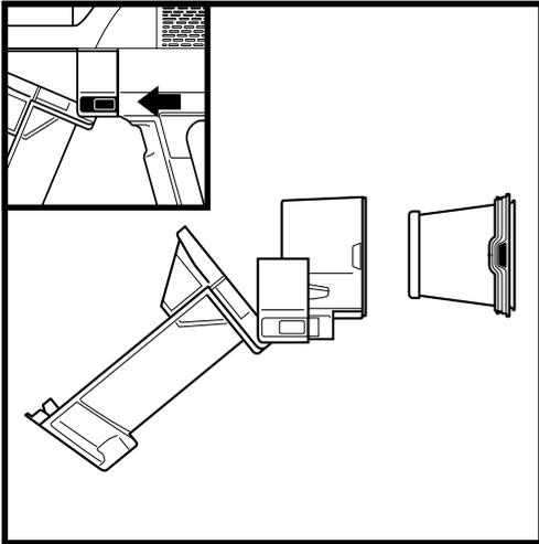
With the dust cup open and the power off, press both release buttons and slide the dust cup out of the hand vac.
