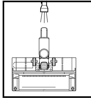
Checking for Blockages in the Floor Nozzle:
