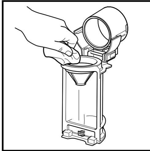
To deep-clean the dust cup, slide the release button until the lid opens completely. Wipe away any dust and debris with a dry cloth, then rinse it out with water. Use a damp cloth to remove any remaining debris. Allow the dust cup to air-dry completely for at least 24 hours before reinstalling it.
