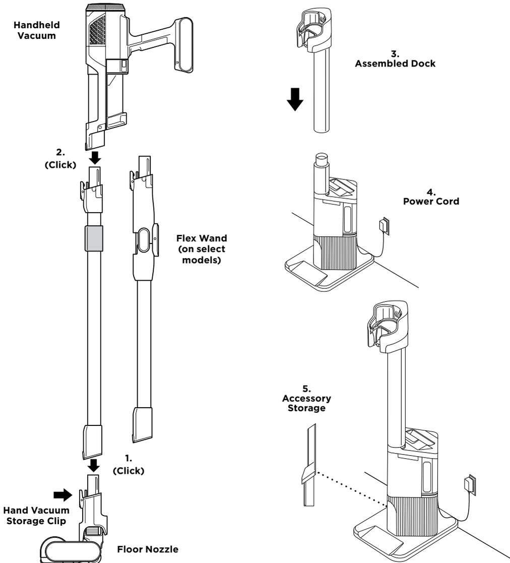
**NOTE:** Once the charging post is installed, it can't be removed.
