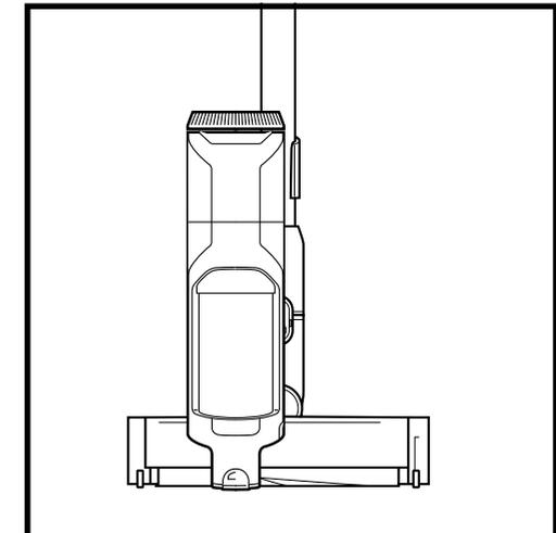
For quick and easy short-term storage, attach the hand vacuum to the wand by placing it onto the pre-assembled wand storage clip.
