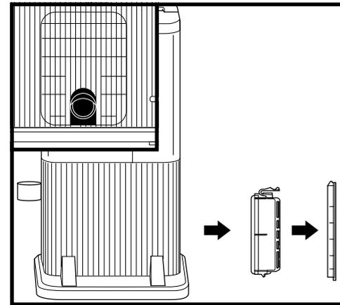
To access the filter in the dock, remove the Filter Door. Press the button at the bottom of the door, then tilt the door and lift it off. Remove the filter from the dock. After the filter has been rinsed and dried, reinstall it by reinserting it into the dock and replacing the filter door.
