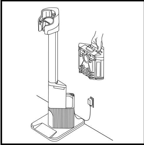
The dock dust bin holds up to 30 days' worth of dust and debris. To remove the bin, press the dust bin release button and lift the bin out by the handle.
