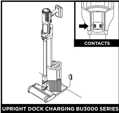
Charge the unit by placing it on the dock. Make sure the contacts on the wand are aligned with the contacts on the charging post. When charging is complete and you need to use the unit again, lift it off the dock.
