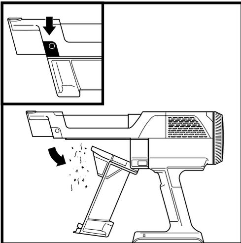
To empty the handheld vacuum dust cup, turn off the power and hold the hand vac over the trash. Press the release button and the dust cup lid will drop open, releasing debris.
