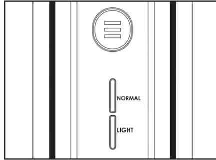
2. Once plugged in, the mop will be in Standby mode and both steam setting lights will blink. Press the Mode Button to select Light or Normal mode, then wait 20 seconds to allow steam to release.
