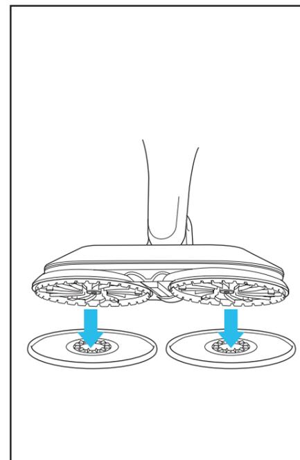
2. To attach the **Dirt Grip Soft Scrub Pads**, place **BOTH** pads flat on the floor with plastic rings facing up. Align the unit directly over the plastic rings on the pads. Gently lower the **Mop Head** onto the pads, pressing until the pads are secure.
