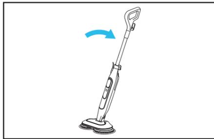
3. Tilt the handle back to activate the spinning pads and begin scrubbing.
