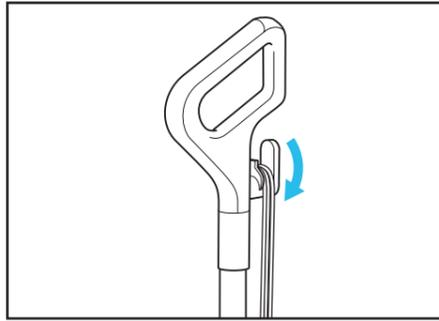
1. Twist the quick-release cord holder to unwrap the power cord completely. Plug into an electrical outlet.
