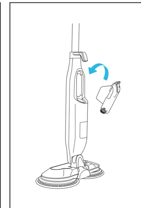
4. When the tank is filled, reinstall it by inserting it back into the mop body.
