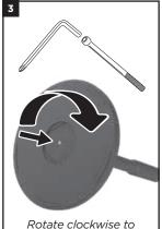
Insert the **Bolt** in the bottom of the Base. Use the Allen Wrench to turn the bolt clockwise to fasten it to the assembled pole.
