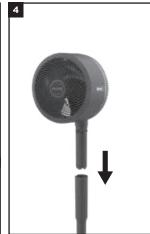
**CAUTION:** finger pinch risk. Holding it by the handle, insert the fan head into the top of the assembled pole until it clicks into place.
