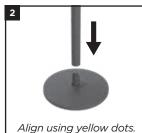
Align the yellow dot on the assembled pole with the yellow dot on the Base, then slide the pole down onto the base.
